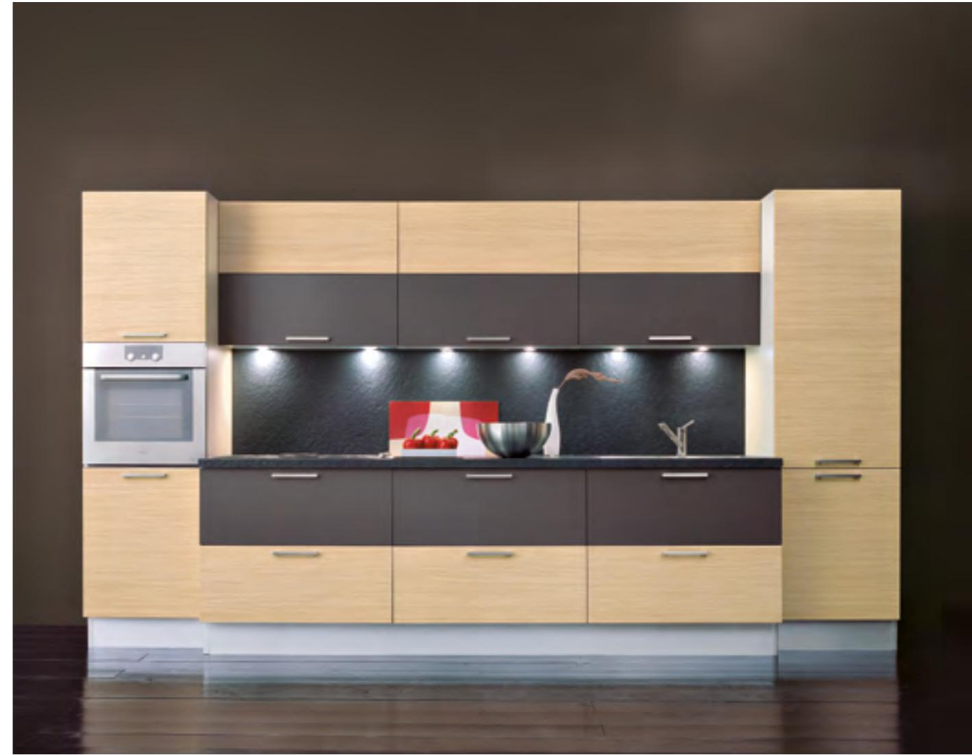
The structure is made of 18 mm particleboard manufactured using E1 rated materials with low formaldehyde emission levels. The particleboards are melamine-coated with a mat finish and doors made of MDF with a white or ecrù polymeric laminate coat and rounded edges. Handles and plinths are made of metal with an aluminium finish. Complete modularity, numerous colour variations. Any design requirement will be met.
